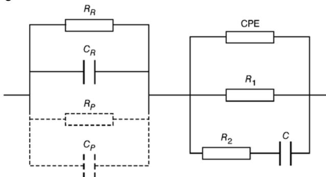
Fig. 2. Equivalent electrical circuit for skin and acupuncture point
