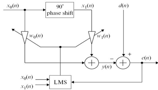
Fig. 3. The structure of adaptive notch filter
