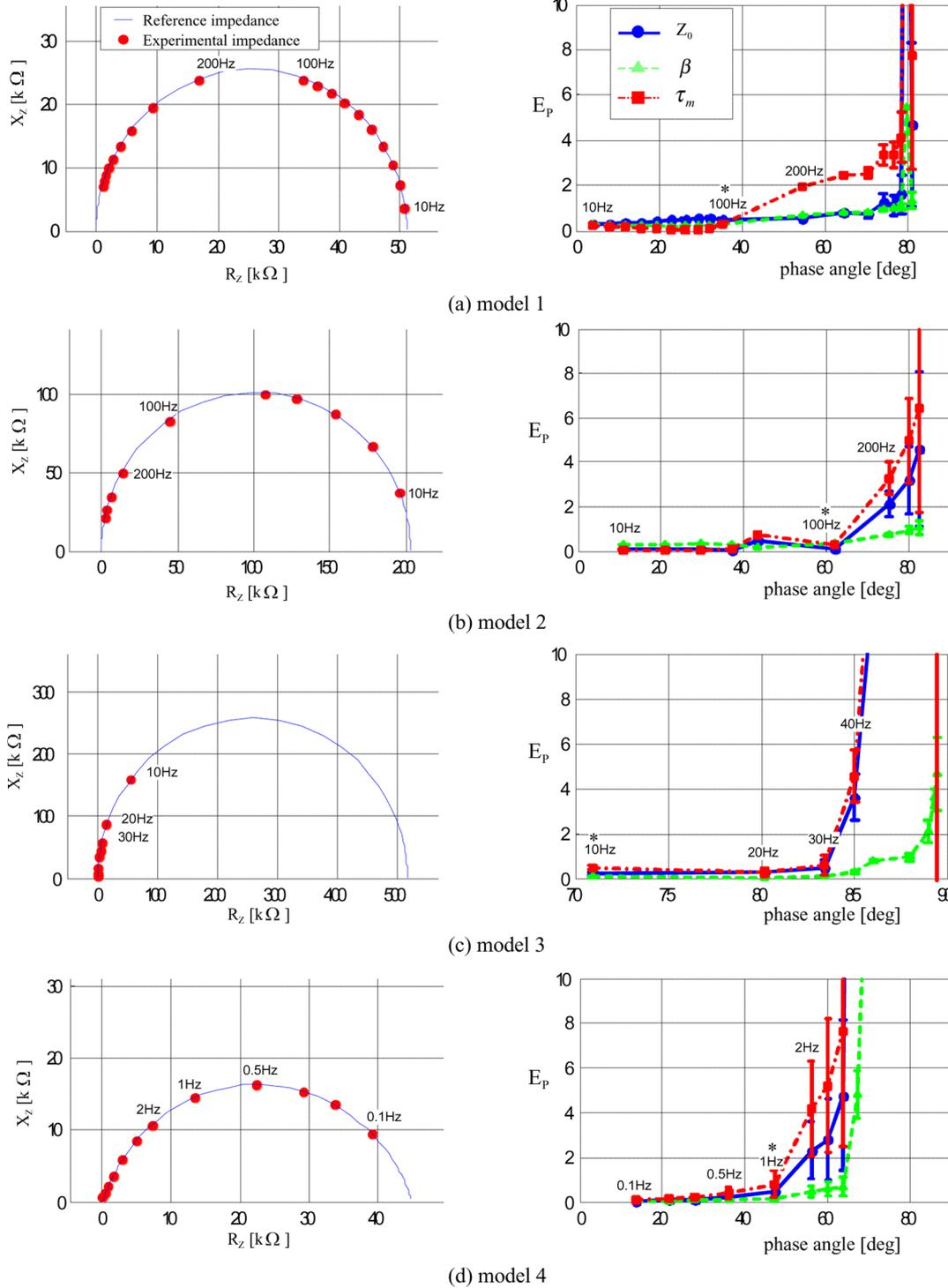
Fig. 3. Test results of the low- to high-level impedance. Left: Impedance locus, right: Parameter estimation error where the basis frequency as high as possible is indicated by \*. See text for the details.
