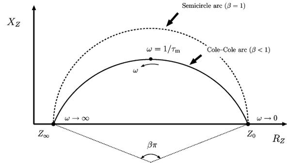
Fig. 1. General impedance locus and corresponding impedance parameters. Note that  $Z_0$ ,  $\tau_m$ ,  $\beta$ , and  $Z_\infty$  indicate the dc resistance, the central relaxation time, the deviation from Debye type ( $\beta = 1$ ) semicircle, and the impedance at infinite frequency, respectively.
