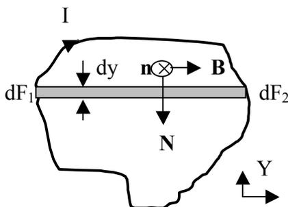
$$\vec{N} = \int I[\vec{n}, \vec{B}]d\vec{S} = I[\vec{n}, \vec{B}] \int d\vec{S} = I[\vec{n}, \vec{B}]\vec{S} = [(IS\vec{n}), \vec{B}] = [\vec{p}_m, \vec{B}].$$
